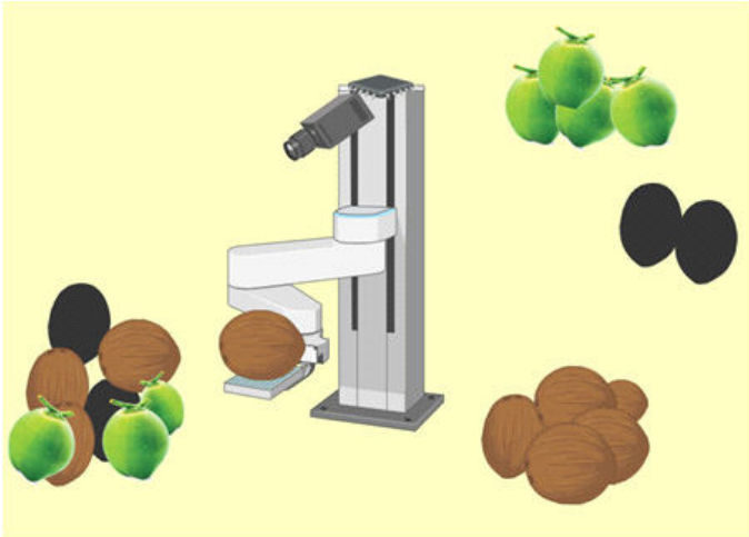
Fig. 2. Proposed concept of stationery coconut grading system
